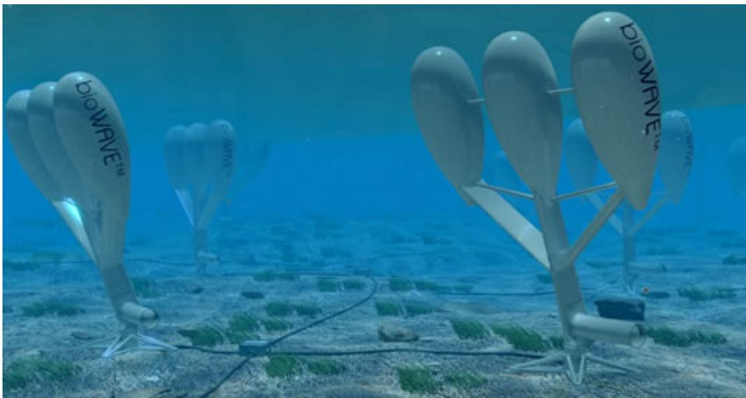
Due to the single point of rotation, this device can align with the flow in any direction, and can assume a streamlined configuration to avoid excess loading in extreme conditions. Systems are being developed for 500kW, 1000kW and 2000kW capacities to match conditions in various locations.”
